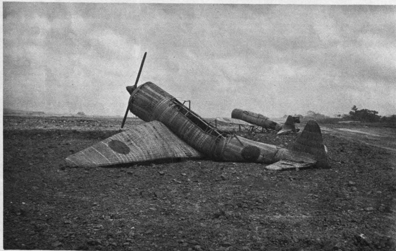
Zeke's tail has been reproduced with amazing accuracy in this rattan-bamboo dummy. Decoy in the background has a fairly convincing cockpit cover and both have the Japanese meatball painted on wing and fuselage. They are extremely difficult to spot from a distance.
